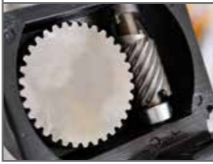
Centrifuge Gear Metal Centrifuge Gear With brake system
